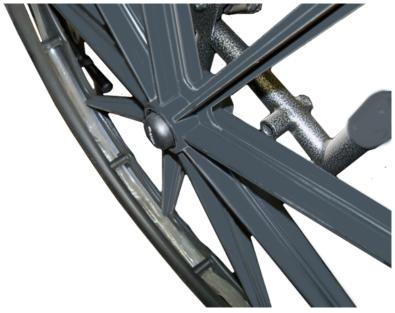
5. With the rear wheels in the hemi position the brakes will have to be adjusted because they will be too hard to apply. Loosen the bolt that holds the brake onto the frame of the chair and move the brake forward about  $\frac{1}{4}$ ".
