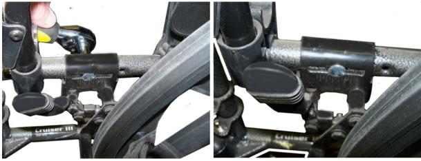
6. Tighten the bolt that holds the brake onto the frame of the chair. Test the brake and adjust if needed. Repeat for the other brake.
