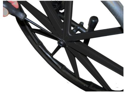
3. Remove the rear wheel with the axle from the lower axle mounting hole and insert the axle in the upper axle mounting hole.
