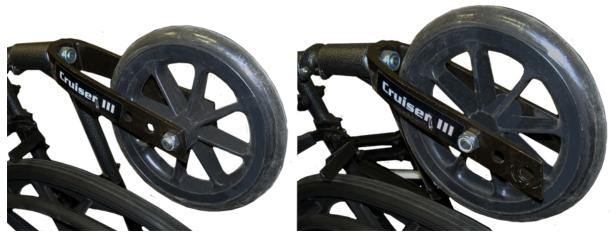
2. Pry the rear axle hub cap off the rear wheel, if so equipped, and remove the rear axle nut.
