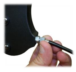
4. Tighten the brake cable adjustment locking nut against the brake handle housing.
