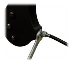
3. Turn the hand brake adjuster counterclockwise to tighten the brake or clockwise to loosen the brake.
