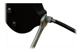
5. If further adjustments are need the same procedure can be made at the lower cable adjuster. Loosen the brake cable adjustment nut away from the frame.
