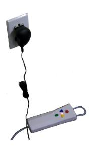
4. The light on the hand control will be red and turn green when finished. This will take about four hours. A charge will last up to six cycles depending on the weight of the person and condition of the battery. By charging the battery after each use the battery will be maintained at its fullest potential.
