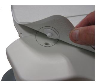
20. After the battery is fully charged disconnect the bettery oberger. Plug the hand control into the rear of the backrest. Make sure the plug is fully engaged.
