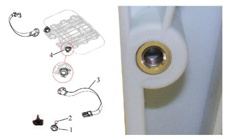
To install accessory number 4, the chest harness. Install one of the nuts (2) onto one of the knobs (1). Run the nut to the end of the knob. Slide the knob through the end of one of the halves of the chest harness (3). Then screw the knob partially into the clamp (4). Position the clamp on the back rest (5) at the desired height. Tighten the knob to lock it into place. Tighten the nut against the chest harness mount.
